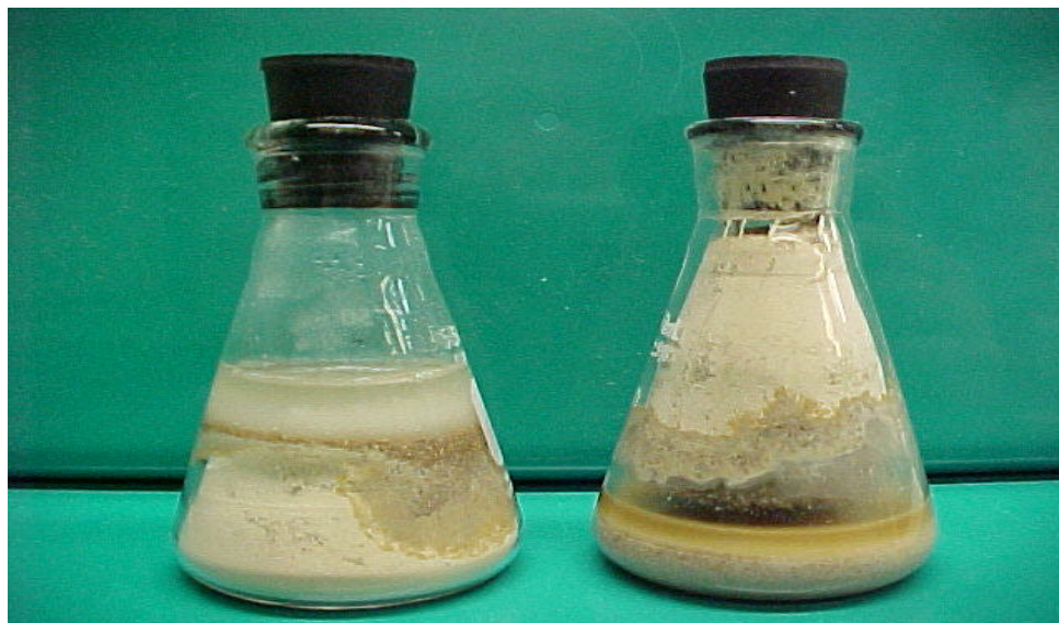
Figure 4. 100 ml Flasks with Scrub absorbed onto Calcine (left) and Calcine absorbed onto Scrub (right).
