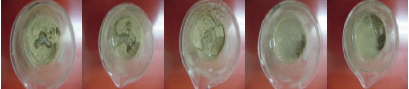
100-ml beakers of 3, 5, 10, 15 and 20 wt% loading of scrub absorbed onto calcine before testing.
