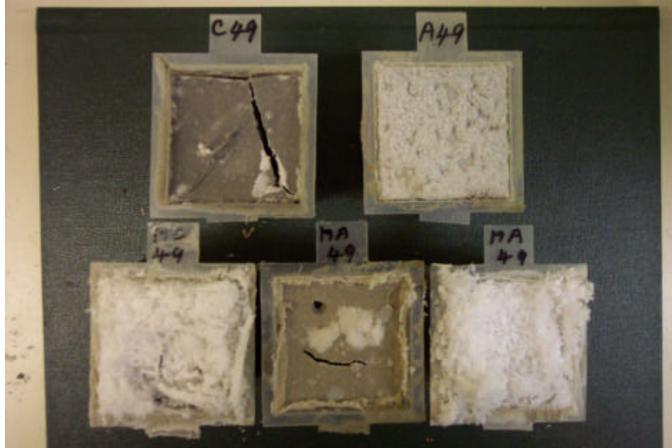
Figure 7. Grout cubes of SBW-189, (A49) and SBW-180 (C49) after neutralization by NaOH. Note the large dimensional changes due to shrinkage, cracking and white sodium nitrate crystallite formation on the surface.
