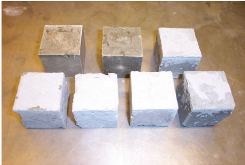
Figure 8. Cured grouts of SBW-189. Left to Right : Top row: A12, A13, A40, Bottom row: A41, A42, A43, and A44. Surface whitening to varying degrees, caused by formation of about 1 mm thick sodium nitrate crystallite layer due to differences in the formulation. Compositions are shown on the formulation diagram Figure 3 and Table 6. Introduction of higher slag content (25 wt%) eliminated sodium nitrate vaporization and crystallization in grouts A12 and A13, and also imparted a brownish color to the grout matrix. Properties of these grouts are shown in Tables 7 and 8, and Figure 6.
