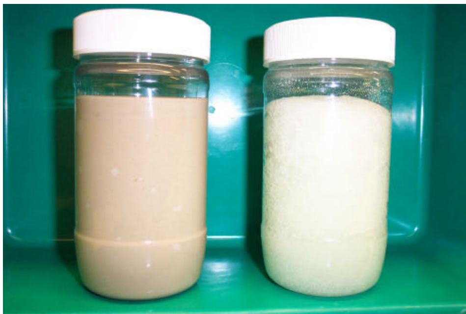
Figure 12. Typical grout (left) and silica gel (right) bottled samples. Note: Both are with SBW-189 simulant. The silica gel was directly loading with no pre-neutralization. The grout contains high slag with calcium hydroxide.
