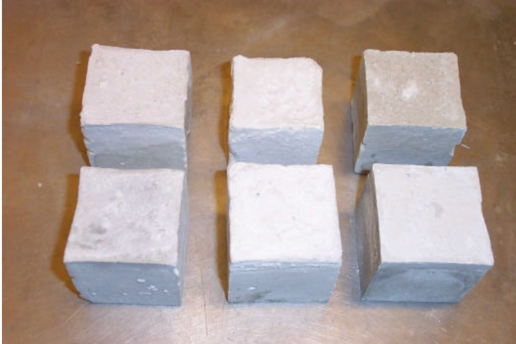
Figure 9. Cured grout of SBW-180. left to right: Top row: C16, C28 and C31, Bottom Row: C41, C43, C44. Properties of these grouts are shown in Tables 7 and 8, and Figure 5. Their relative compositions are shown on the formulation diagram, Figure 4 and Table 6.
