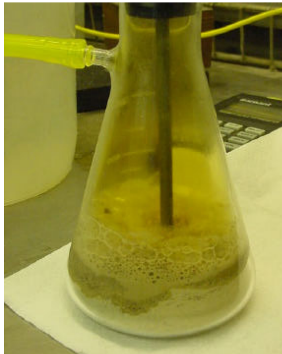
Figure 6. 500-ml Flask showing foaming and NO x when scrub solution and calcine are mixed together.
