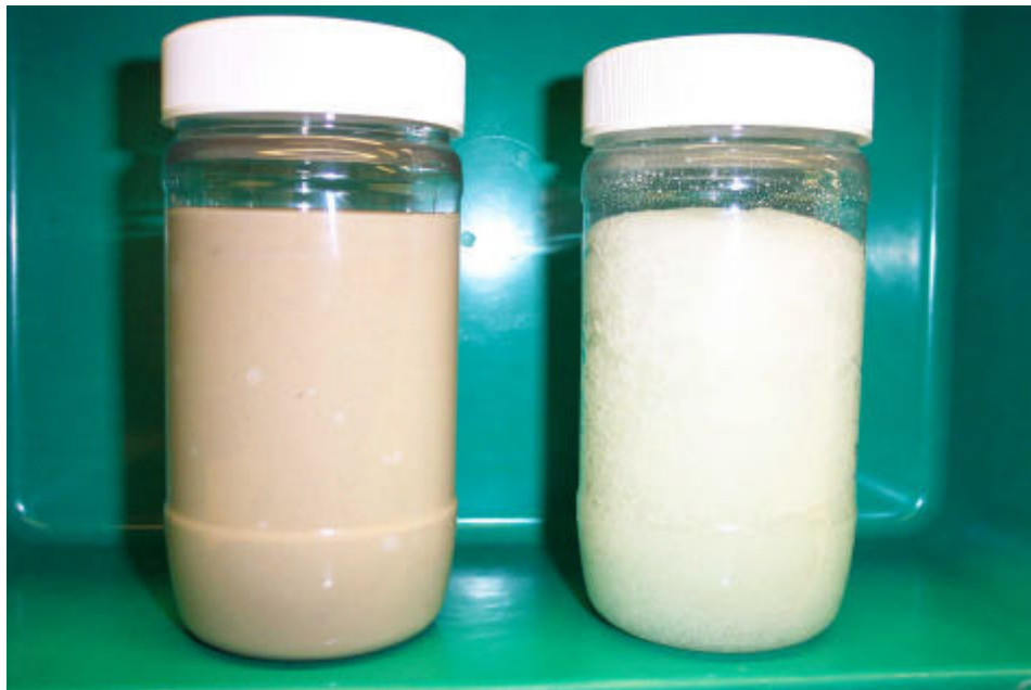
Figure 2. Typical grout (left) and silica gel (right) bottled samples. Note: Both are with SBW-189 simulant. The silica gel was directly loading with no pre-neutralization. The grout contains high slag with calcium hydroxide.
