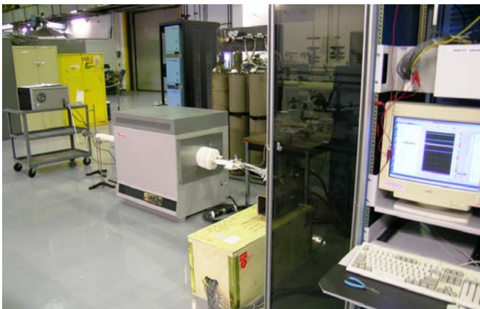
Fig. 7. Long duration 1200 °C thermocouple test setup.
