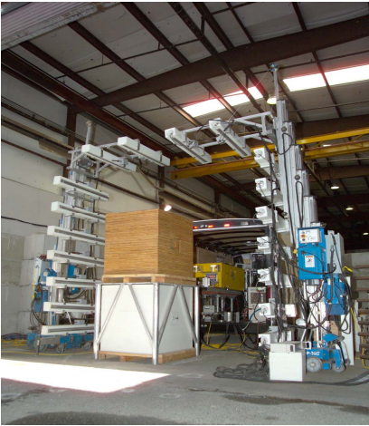
Figure 1. The transportable PPA interrogation system including the Varitron accelerator along with custom neutron and gamma detectors.
