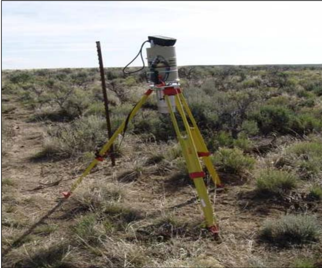
Figure 3. High-purity germanium detector used to measure Cs-137 in soils.
