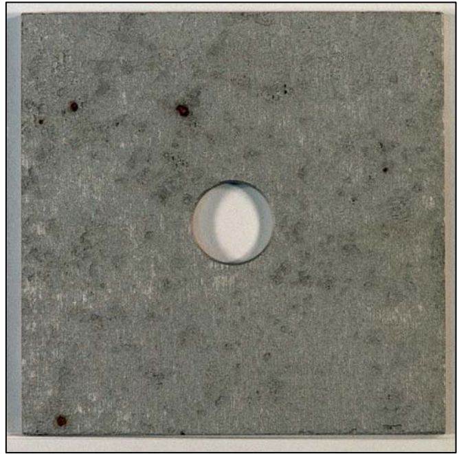
FIGURE 4 - Carbon Steel Coupon After Cleaning, 6-year exposure at 3.05-m
