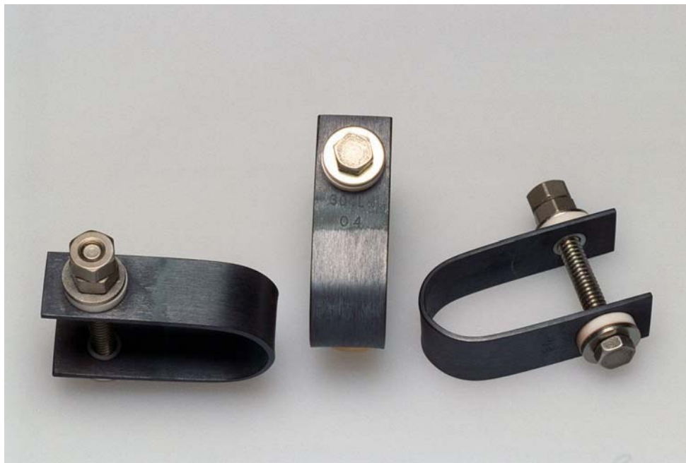
Figure 18. Type 304LW tested in 40-wt% hydroxide solution with halides at 90°C.
