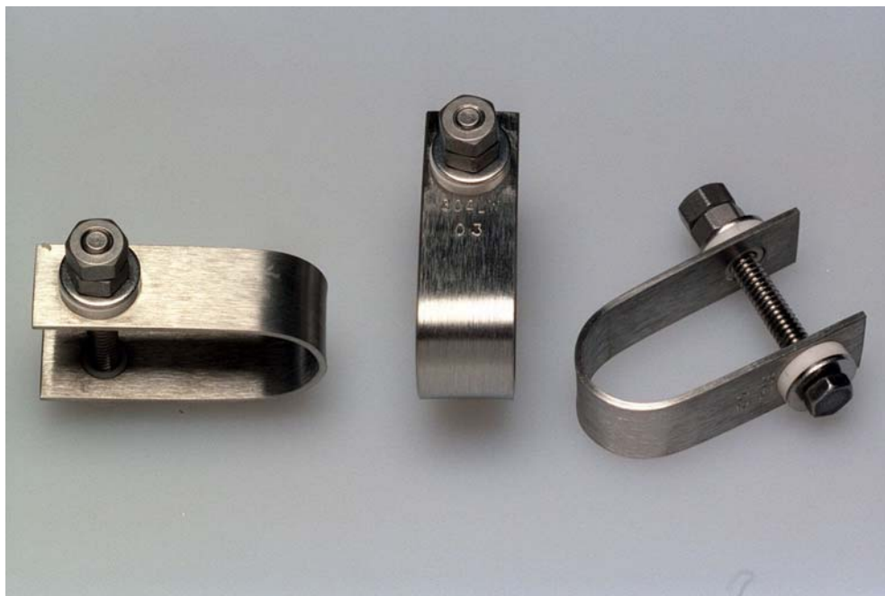
Figure 16. Type 304LW tested in deionized water at 90°C.
