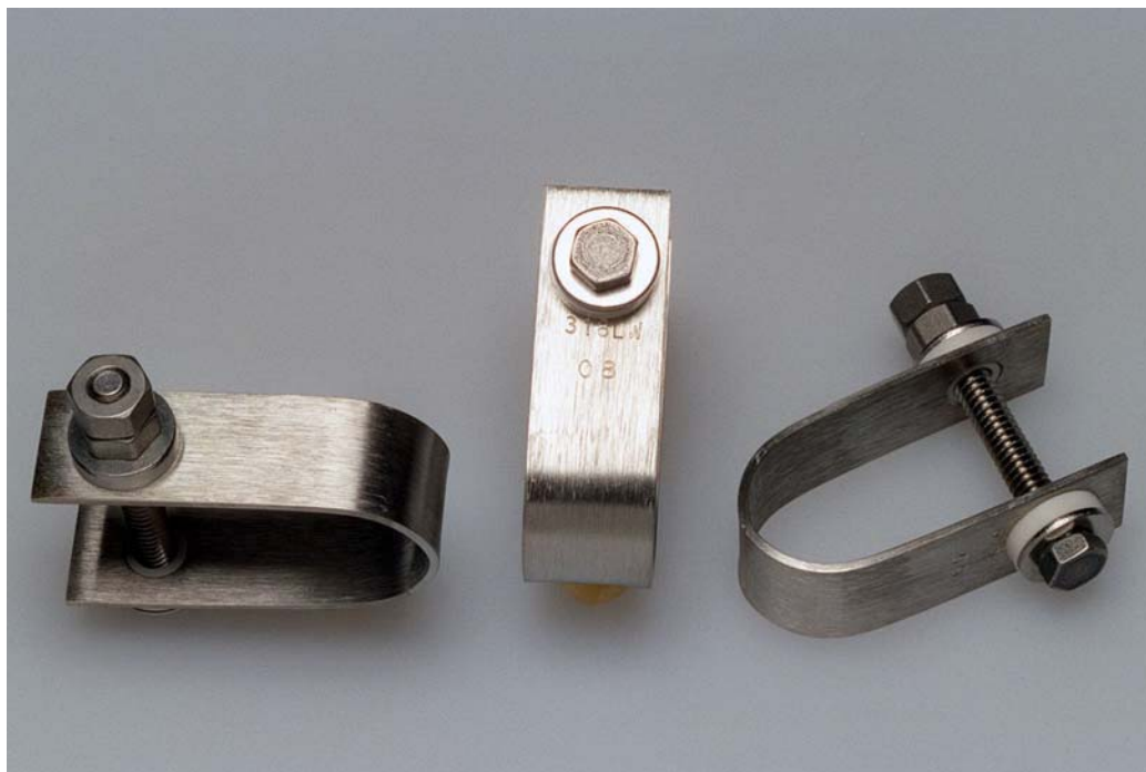
Figure 5. Type 316LW tested in deionized water at 90°C.
