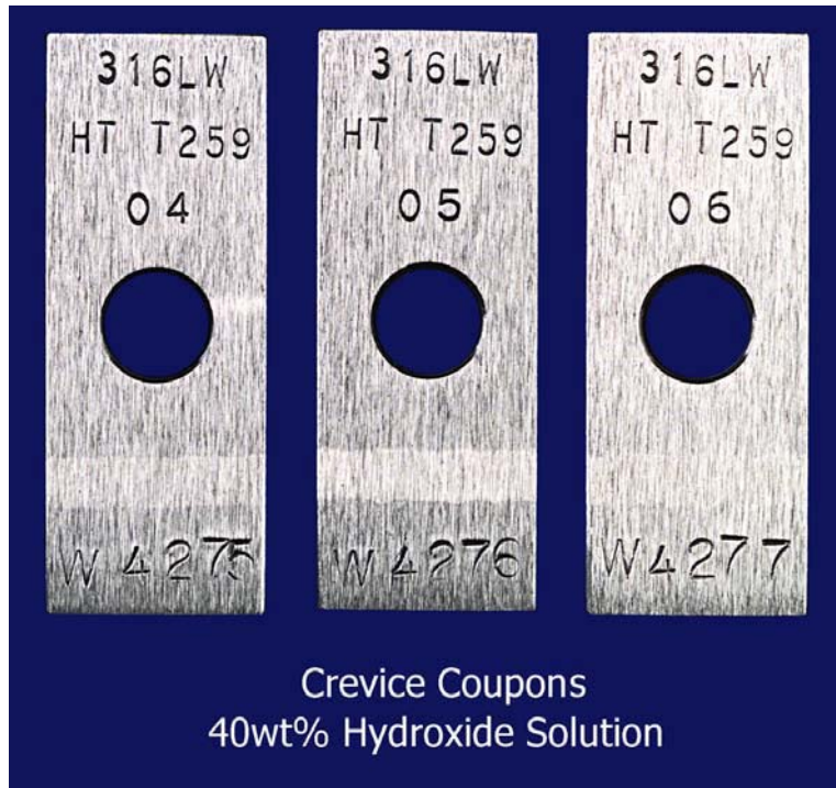
Figure 3. Type 316LW tested in 40-wt% hydroxide solution with halides at 90°C.
