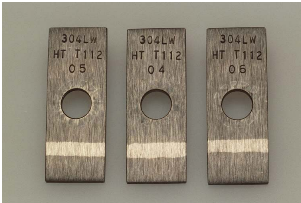
Figure 14. Type 304LW tested in 40-wt% hydroxide solution with halides at 90°C.
