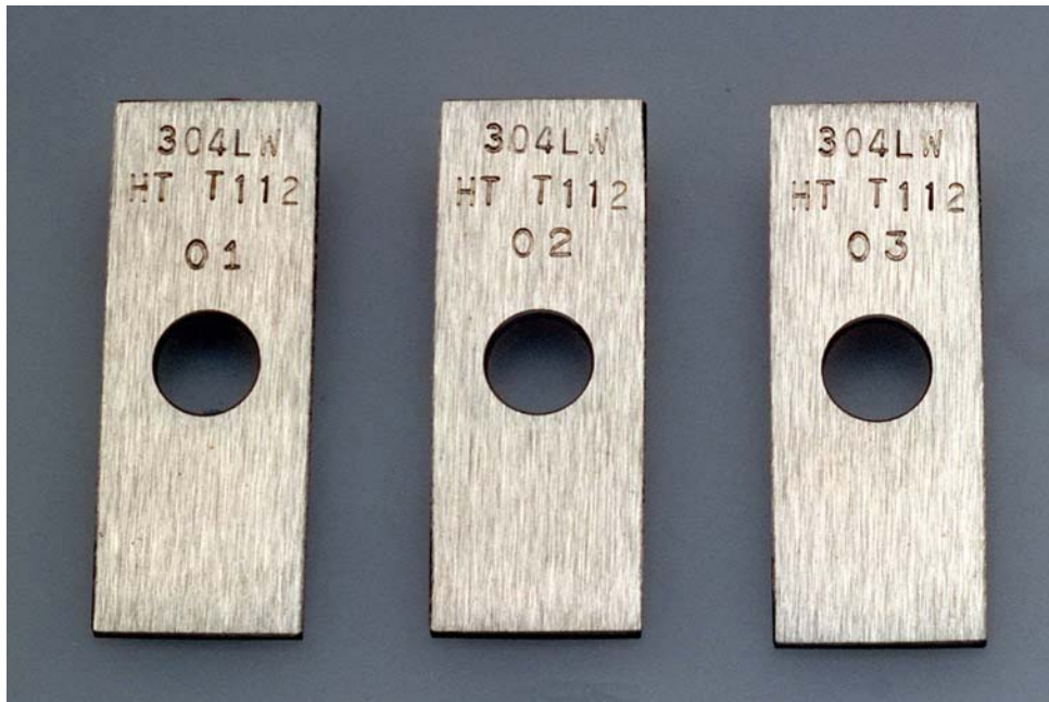
Figure 12. Type 304LW tested in deionized water at 90°C.
