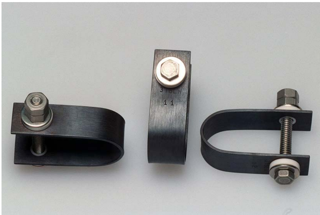
Figure 9. Type 316LW tested in 40-wt% hydroxide solution without halides at 90°C.
