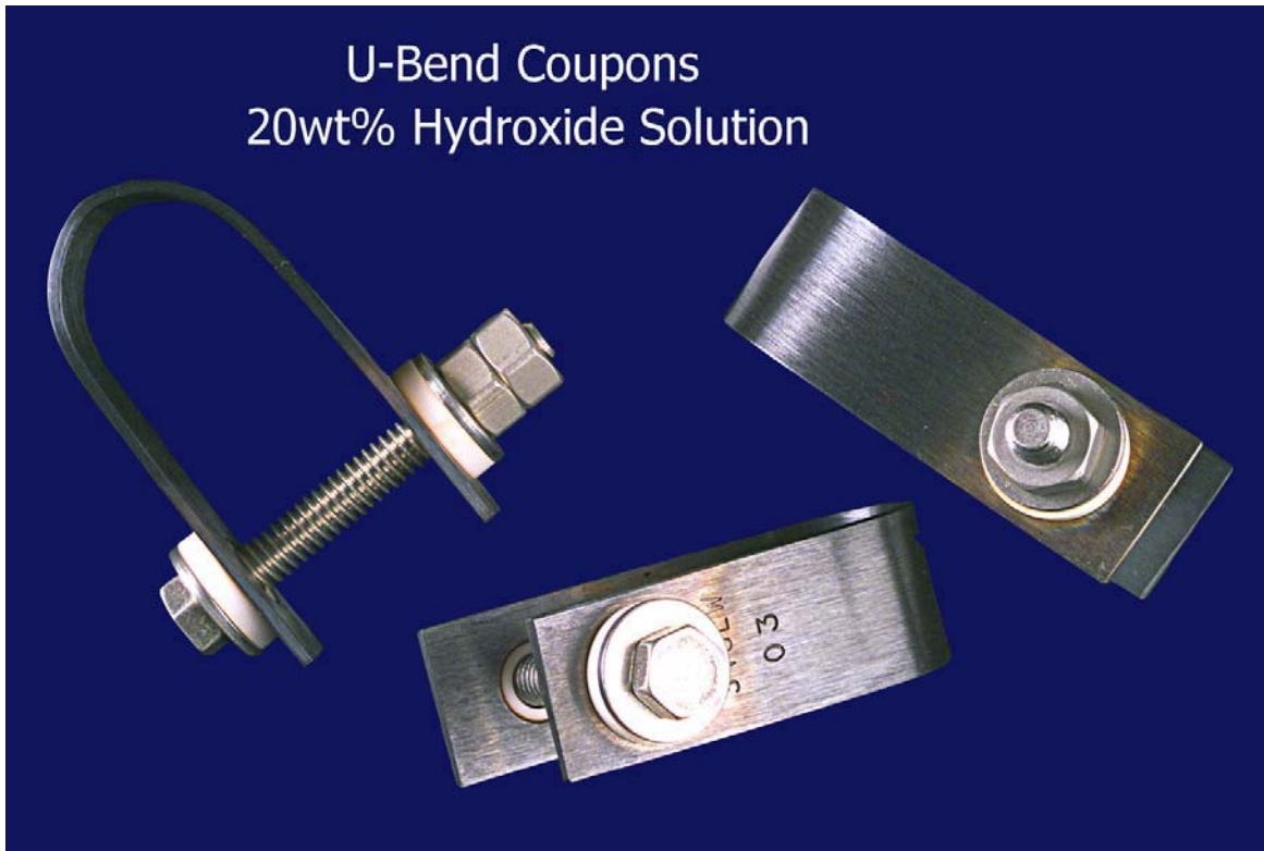
Figure 6. Type 316LW tested in 20-wt% hydroxide solution at 90°C.
