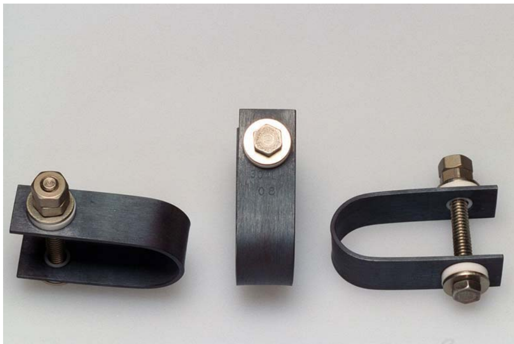
Figure 19. Type 304LW tested in 40-wt% hydroxide solution without halides at 90°C.
