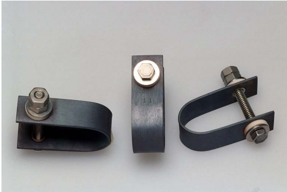
Figure 17. Type 304LW tested in 20-wt% hydroxide solution at 90°C.
