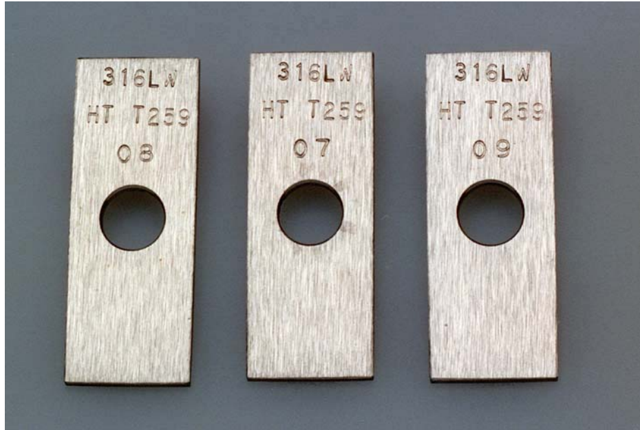
Figure 1. Type 316LW tested in deionized water at 90°C.
