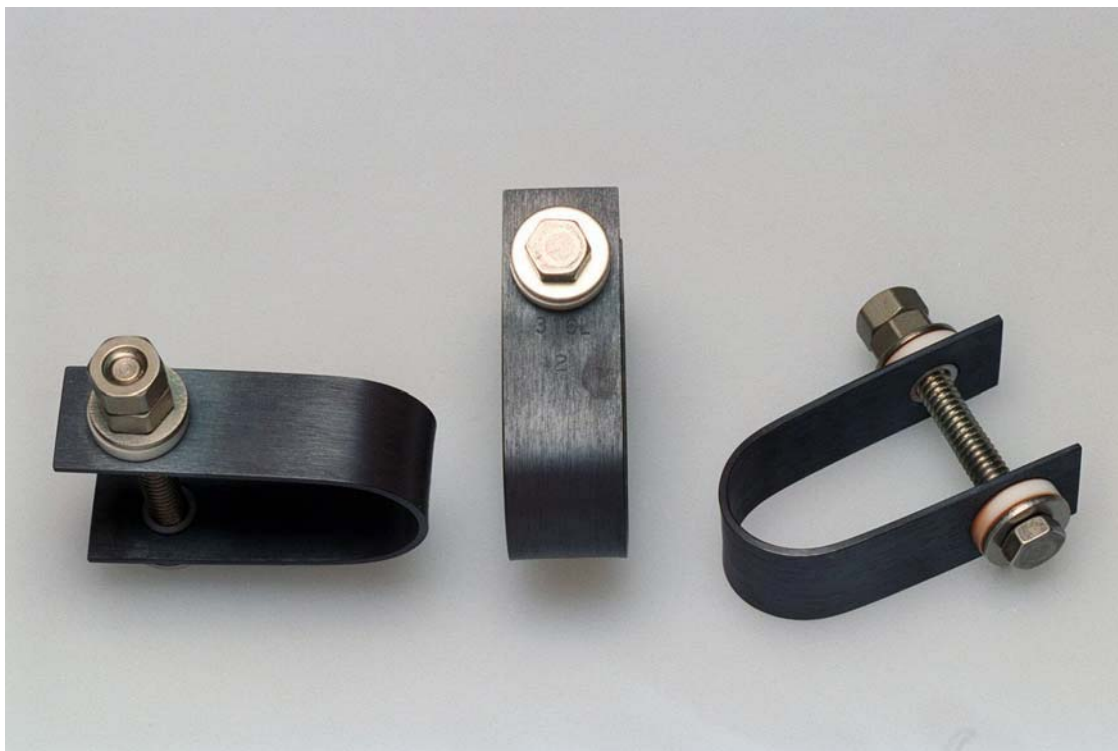
Figure 10. Type 316L (unwelded) tested in 40-wt% hydroxide solution with halides at 90°C.
