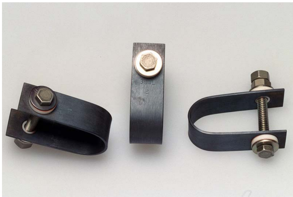
Figure 20. Type 304L (unwelded) tested in 40-wt% hydroxide solution with halides at 90°C.
