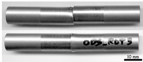
Figure 8. Typical torsional mode weld, illustrating results of fixture misalignment. Axial load 300 N (~67 lbf), torsional motion +30°, -60°, +30° over 2 s, temperature 850°C.
