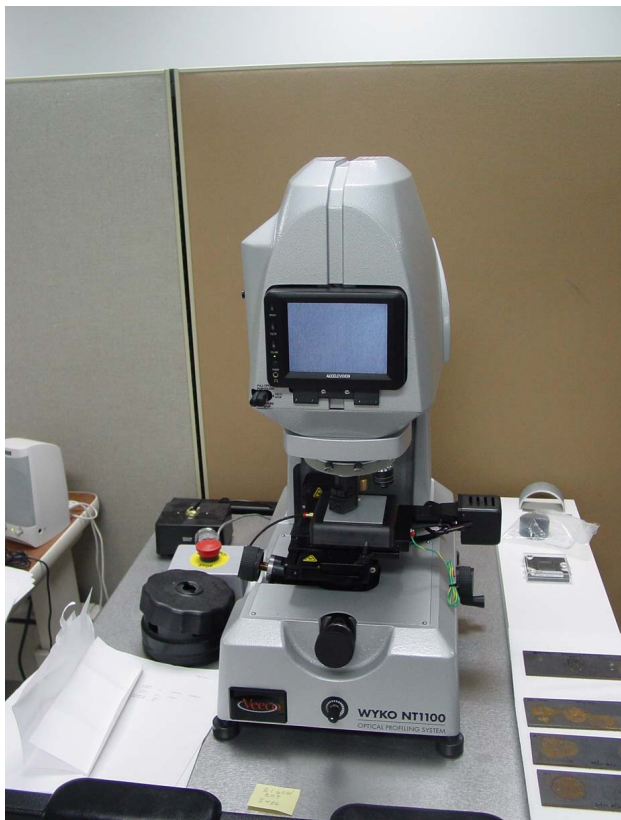
Fig. 2. Wyko Model NT1100 Optical Profiler used to obtain surface roughness measurements.
