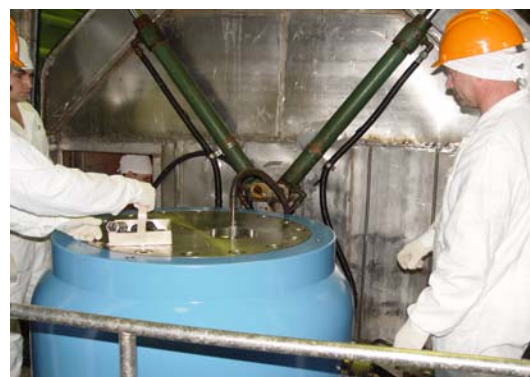
Figure 10. Mayak technicians depressurizing before opening the VPVR/M cask lid.
