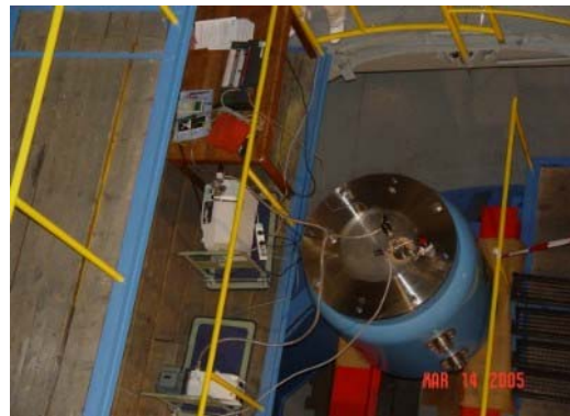
Figure 6. VPVR/M cask leak test demonstration.
