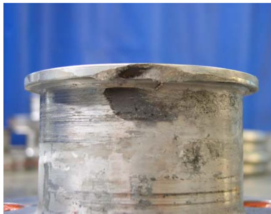
Figure 14. Cask trunnion wear resulting from loosening of the tiedown system during transport of the VPVR/M cask between NRI in Rez and Mayak in the Russian Federation.
