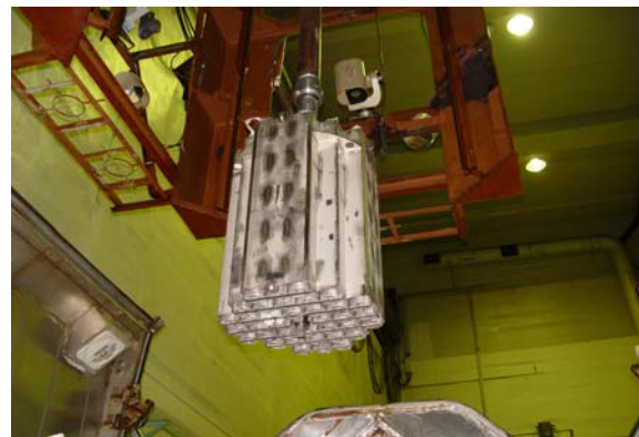
Figure 4. Basket being lifted out of the cask using the central suspension/hanger.
