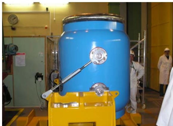
Figure 7. VPVR/M cask secured in vertical position on cask manipulation frame.
