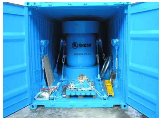
Figure 12. SKODA VPVR/M cask and ancillary equipment.
