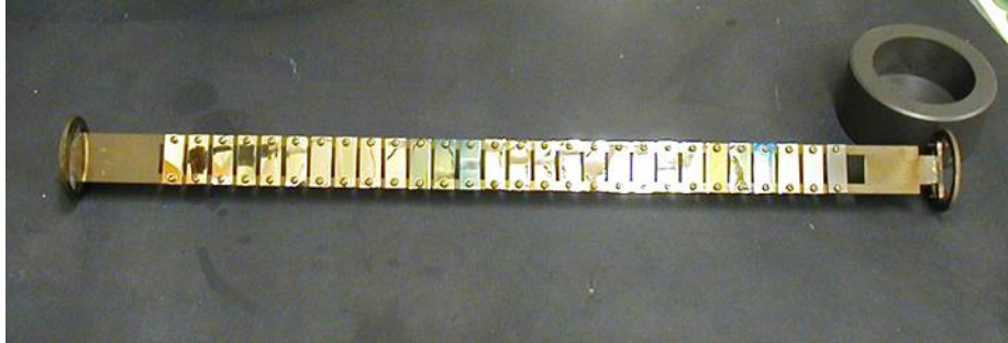
Figure 101 Inconel 625 holder used for fixturing the samples in the SCW corrosion cell. The test samples were 1.25" in length, 0.5" in width, and about 0.02" in thickness.
