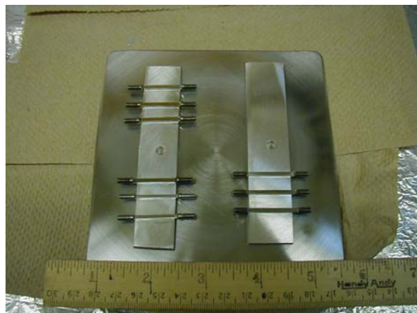
Figure 128 SCC samples of the three steels, HT9, HCM12A and T91 steels just after removing from the plasma immersion ion implantation chamber after oxygen ion implantation.
