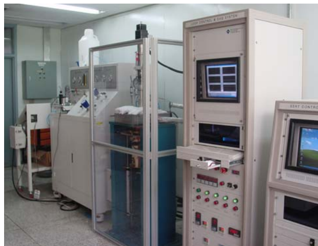
Figure 90 SCW SCC Test Loop at KAERI (1).
