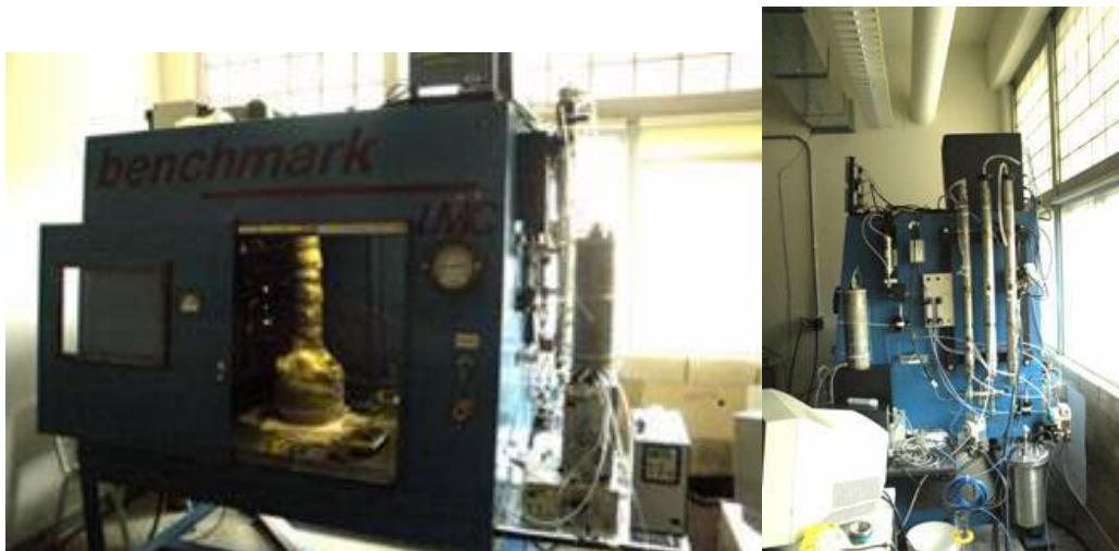
Figure 100 Supercritical water corrosion cell at the University of Wisconsin, used for the 600oC SCW corrosion tests.
