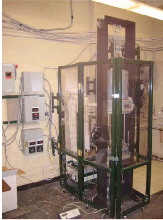
Figure 47 Photograph of the multi-sample SCW-SCC facility in HTCL.
