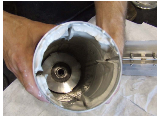
Fig. 4. Solids capture, inside rotor.
