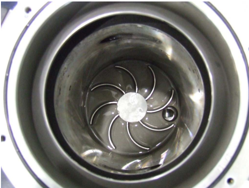
Fig. 11. Following CIP, mixing plate.
