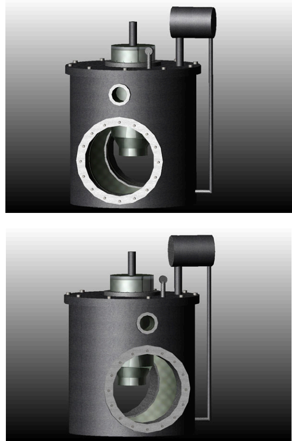
Figure 1. An Overall View of the SBLB Water Tank with an APR1400 Vessel/Insulation Simulator
