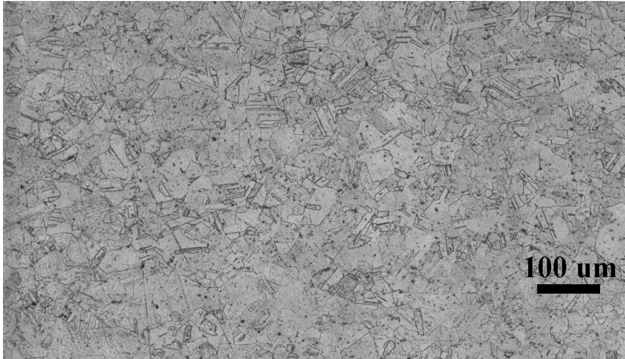
Figure 28 – Photomicrograph showing VPS copper deposit in the as-sprayed condition.
