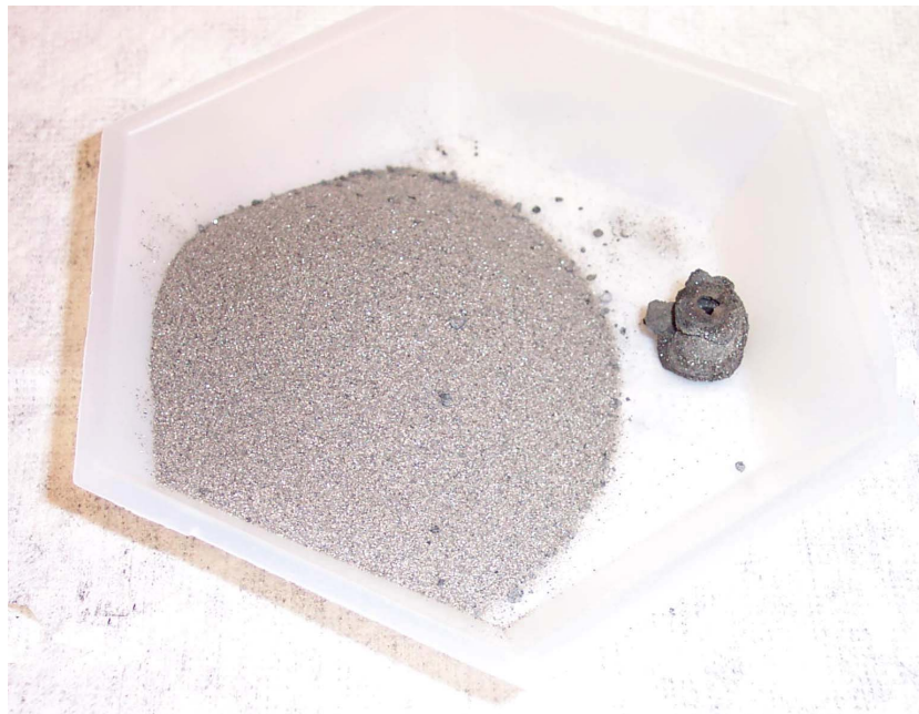
Figure 2. Bed material and nozzle deposit formed during operation with the MAC/DTPA feed..
