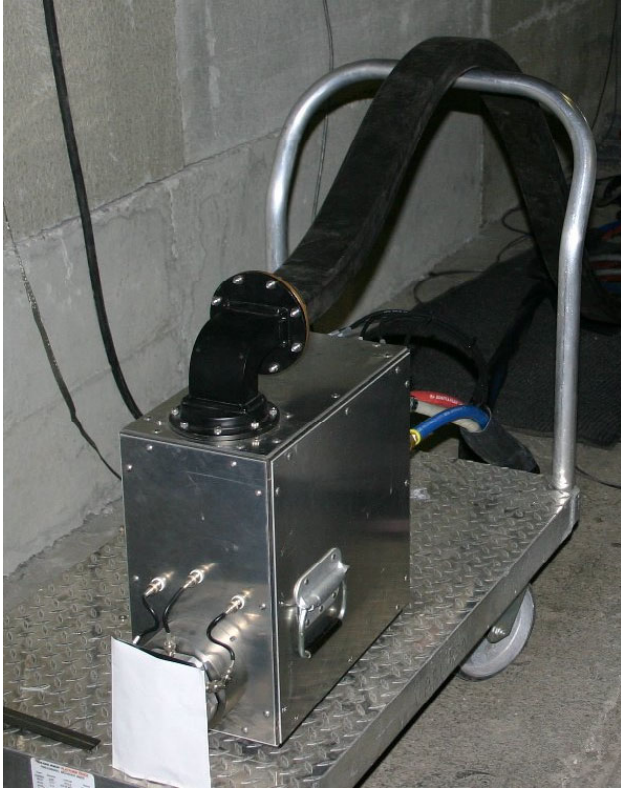
Figure 2. Components used for radiographic testing at the Idaho Accelerator Center Annex in Pocatello, ID. Left: Linear accelerator and waveguide (the paper does not attenuate much radiation!). Right: Rotational stage used for holding and angular positioning fueled clads. A full-scale surrogate is in the clad holder and pieces of another surrogate are at the sides.
