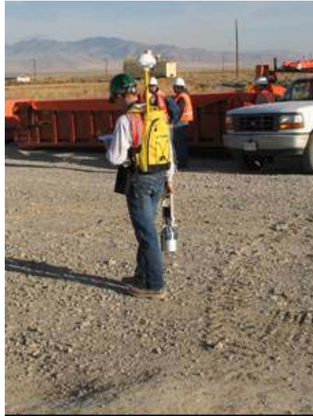
Fig. 1. BaSIS real-time measurement system.
