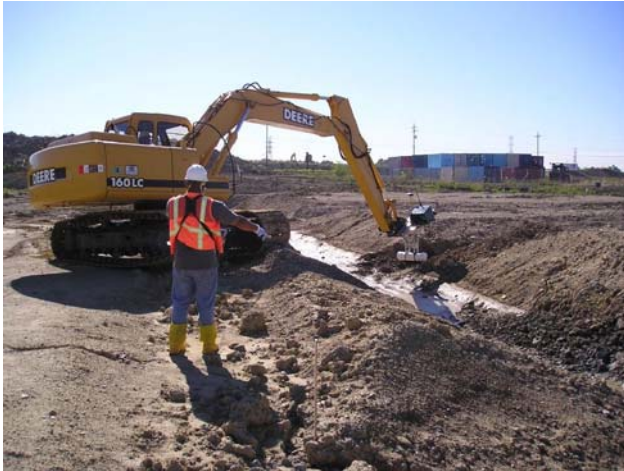
Figure 3. EMS NaI platform used to survey a trench at FCP.
