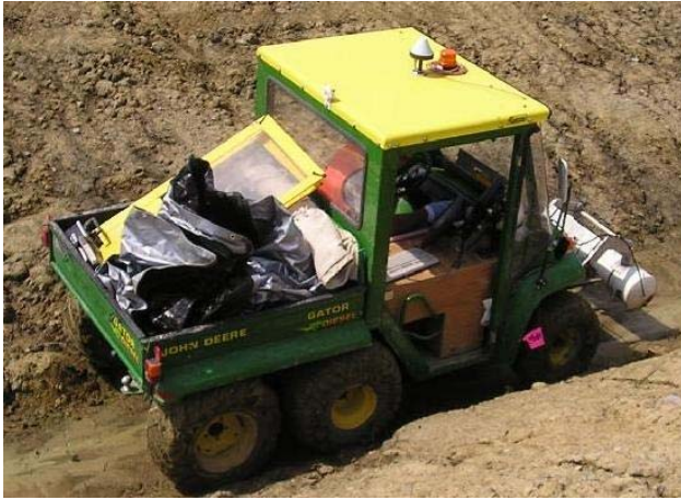
Figure 1. The FCP GATOR platform and front-mounted NaI detector.
