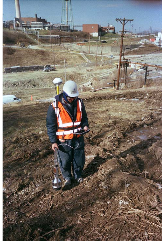
Figure 7. BaSIS survey of hillside at MCP using FIDLER detector.
