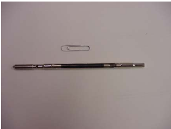
Figure 6. FFTF stainless steel fuel pin containing 0.4 mm diameter UO_2 fuel pellets.
