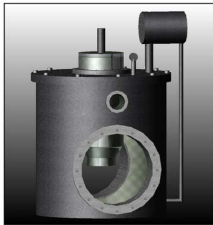
Figure 7. SBLB facility for ERVC testing (test section with insulation). (Cheung, et al., 2003)
