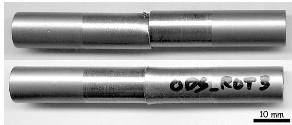
Figure 2. Typical torsional mode weld, illustrating results of fixture misalignment. Axial load 300 N (~67 lbf), torsional motion +30°, -60°, +30° over 2 s, temperature 850°C.
