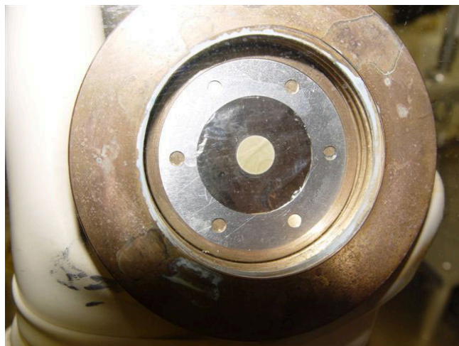
Figure 2. Plutonium-239 target prepared by INL for use in the LANL DANCE array.
