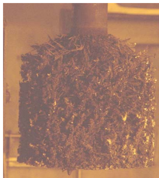
Figure 3. A cathode removed from Mk-IV ER, 10.1 kg
