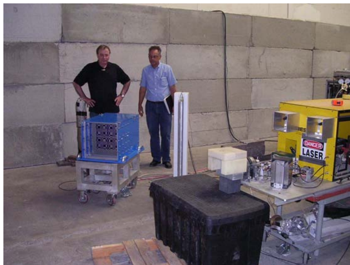
Fig. 5 BNL imaging system and the basic test configuration. The linac is on the right side.
