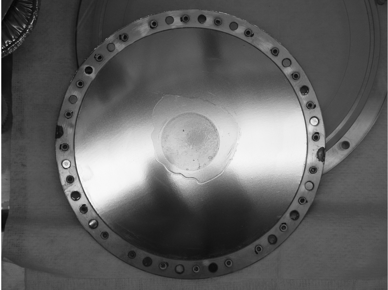
Figure 6. Picture of stainless steel fission foil containing electroplated ^{242}\text{Pu} ( 1086 \pm 54\mu\text{g} ).
