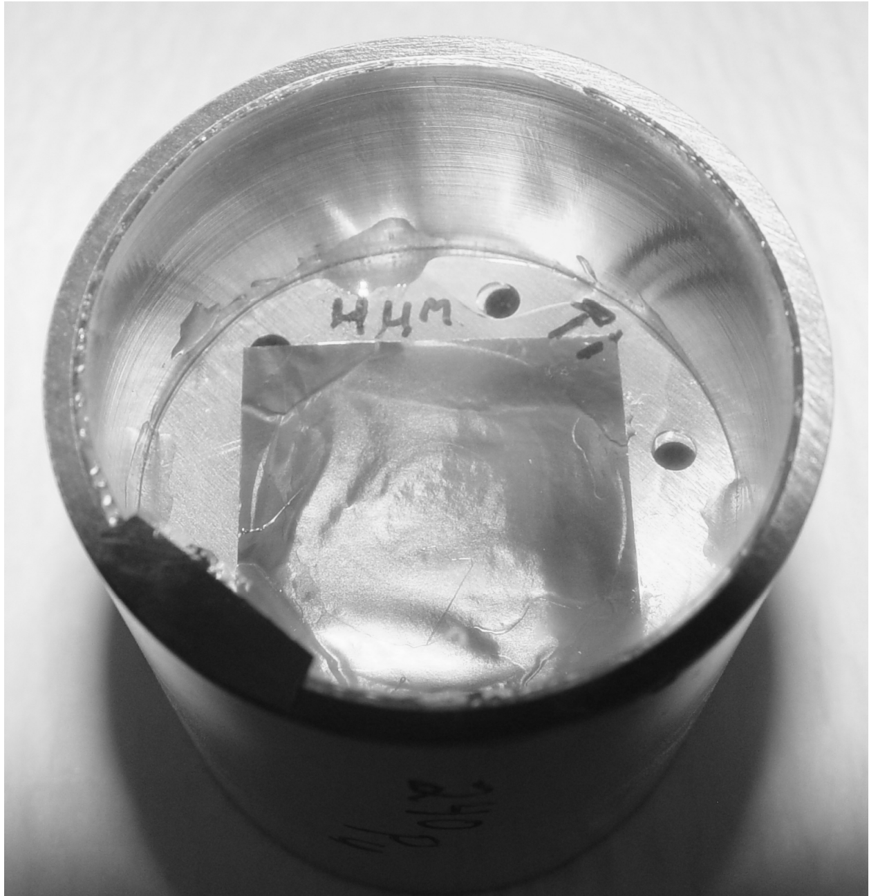
Figure 3. Picture of DANCE Radioactive Target Holder containing ^{240}\text{Pu} target.
