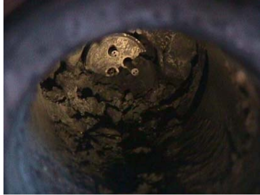
Figure 7 – Failed thermocouple in a gasifier thermocouple port due to shear or slag binding. (Note that slag has infiltrated into the point where the thermocouple failed at the back side of the thermocouple.)
