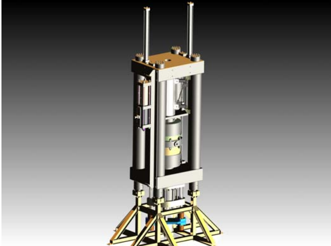
Figure 4. Computer-generated rendering of the UDS to be used at NETL to study deep drilling phenomena.
