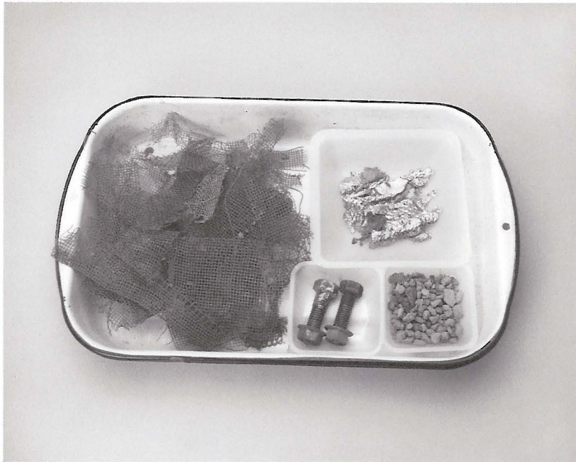
Figure 3. Plain-light image of a representative split of the oversize fractions of shell components after hand-sorting, jaw- and roll-crushing, initial screening and magnetic separation. At top right are typical pieces of titanium-alloy splash. At bottom center are 5-cm (2-inch) bolt and nut sets and at bottom right is the relatively small amount of oversize pieces of refractory that remain after crushing.
