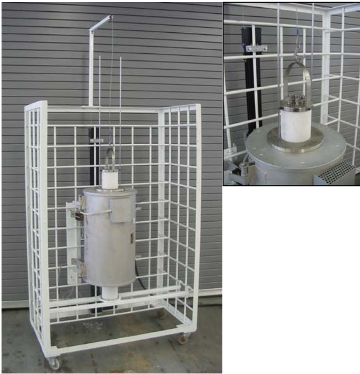
Fig. 2: Cyclic oxidation apparatus for testing in atmospheric pressure steam/air mixtures at up to 800°C.
