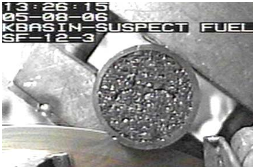
Figure 2.6. Sectioning of SF-12 with Low Speed Isomet Saw. Water is being used a coolant/cutting lubricant. The outside diameter of SF-12 is 0.55 to 0.56 inch. A portion of the circular saw blade is shown below the fuel.
