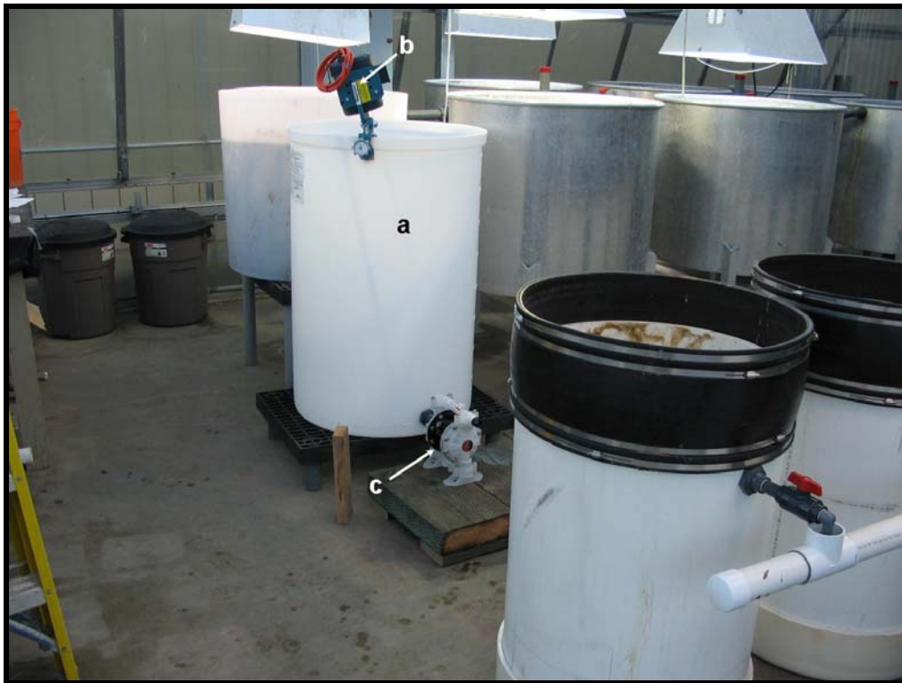
Figure 2 . Slurry mixing and transfer equipment. Components include: a) mixing tank; b) mixer; and c) double diaphragm slurry pump.
