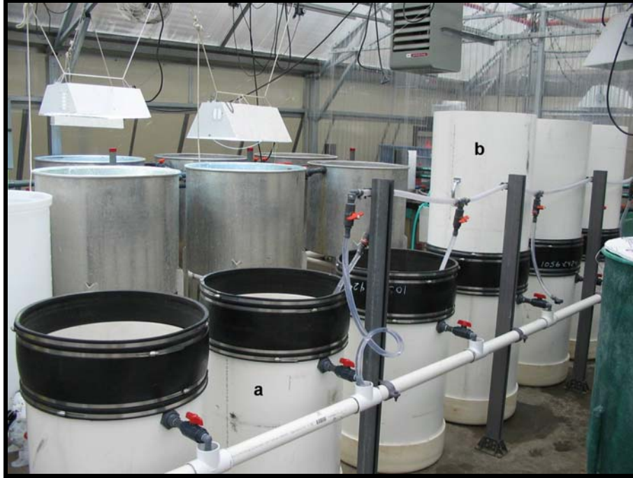
Figure 3. Experimental chambers in various stages of the experiment. Each chamber comprised a lower permanent tank (a) and a removable top section (b).
