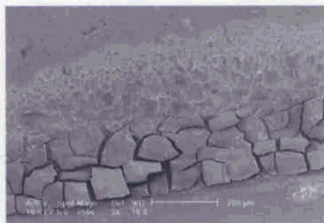
Figure 8: SEM image of corrosion products observed in crevice corrosion tests for Alloy C-22 (8).
