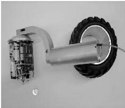
Figure 1. The Smart Wheel with the tire and hub removed
