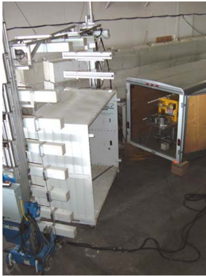
Figure 4. Photographs of the prototype PPA system with a cut away of a cargo container (left), and a metric ton of polyethylene being moved into position for a nuclear material inspection (right).
