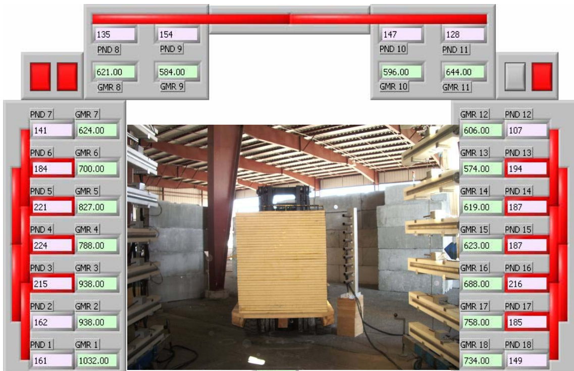
Figure 11. Selected user interface display with a representative Calibration Pallet inspection (while the INL Celotex Calibration Pallet is pictured, the data presented is from a Lead Pallet inspection).
