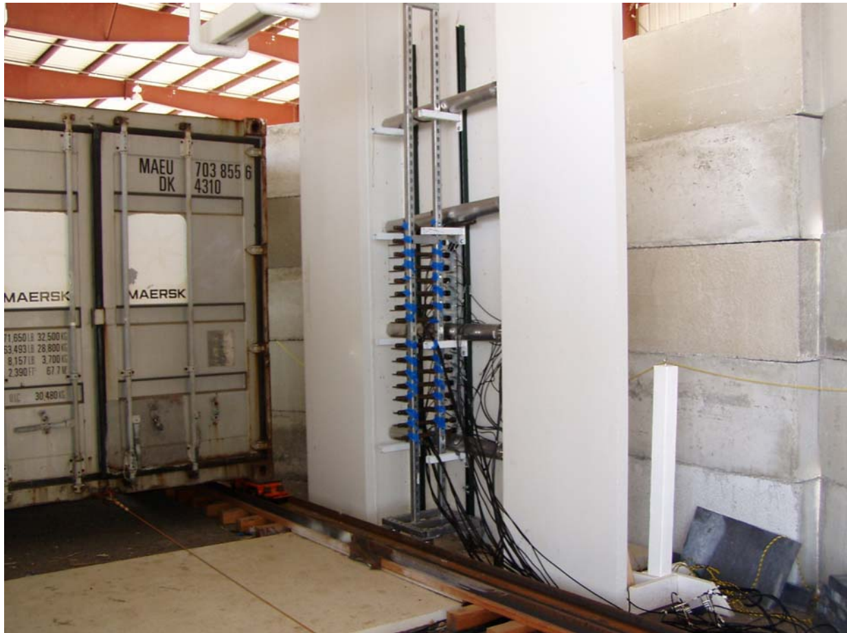
Figure 14. PACECO/ISU/INL gray scale density mapping system mounted with the IAC cargo container translation test assembly.
