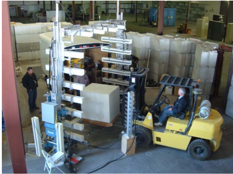
Figure 4. Photographs of the prototype PPA system with a cut away of a cargo container (left), and a metric ton of polyethylene being moved into position for a nuclear material inspection (right).
