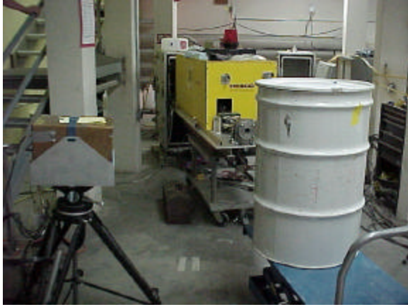
Figure 19. Polyethylene-filled drums used to provide shielding for nuclear material located inside the center hole. [Barrel #2 is shown with its top removed.]
