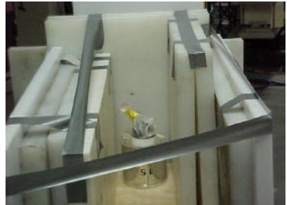
Figure 7. HEU shielded with 10.16 cm (left) and 19.05 cm of polyethylene.
