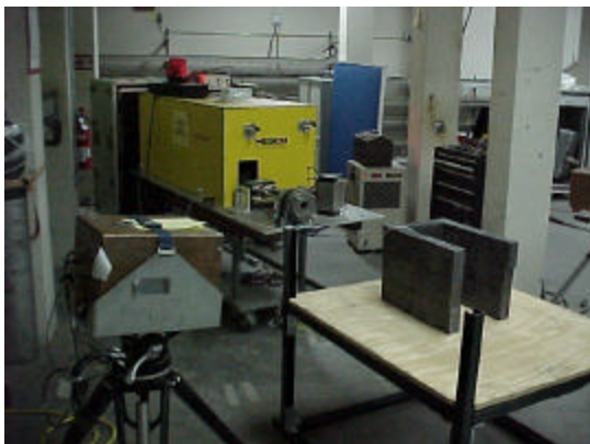
Figure 8. HEU shielded by 5.08 (left) and 10.16 cm of lead.
