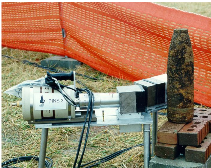
Figure 2: A 4.7-inch artillery projectile during assessment in the Spring Valley neighborhood of Washington, D.C., January 1993. PGNAA determined this “non-stockpile” projectile contains an incendiary chemical. The projectile was likely buried in 1919.
