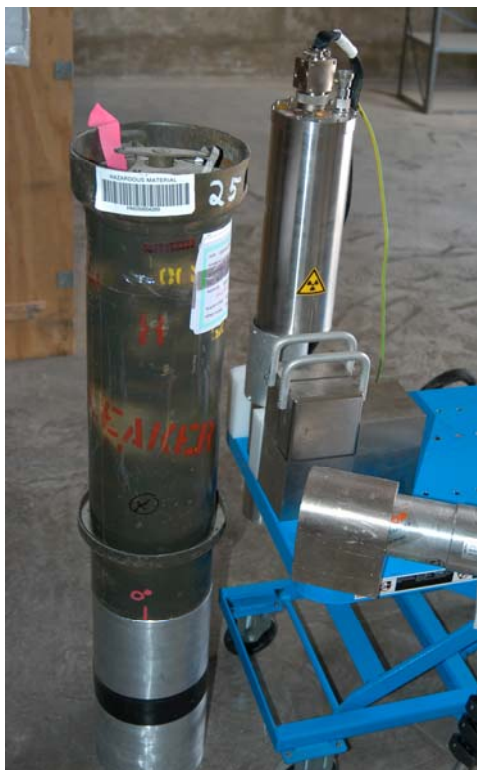
Figure 4: A SODERN neutron generator irradiates a mustard-agent filled 4.2-inch mortar projectile during a test assay at U.S. Army Dugway Proving Ground, September 2003. For safety, the mortar projectile is overpacked inside the air-tight olive-drab steel can stenciled “LEAKER.”
