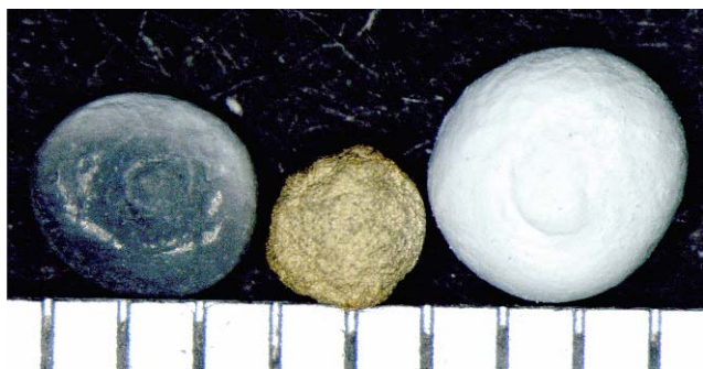
Fig. 4. From left to right, microspheres of a) carbide, b) nitride, and c) oxide.
