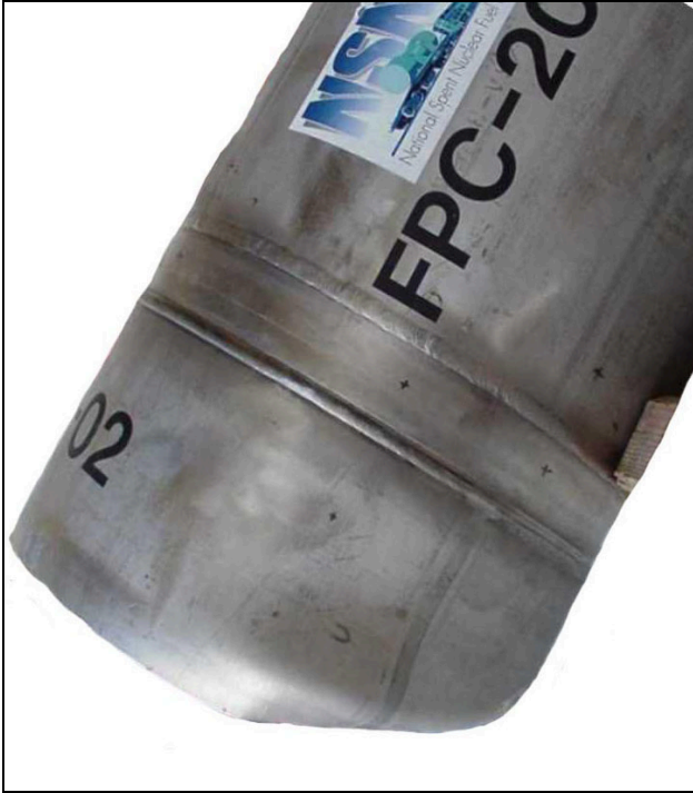
Figure 4. Side View of Deformed Test Specimen (21° Impact Angle)
