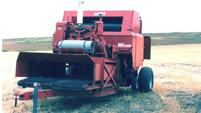
Figure 3. The separate chassis of the single pass multi-component harvester system, attached to a baler.
