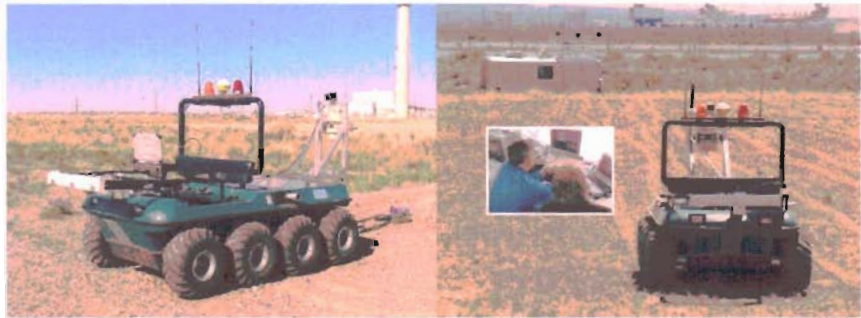
Figure 5: RATV being operated in the field relaying data to the remote control station.
