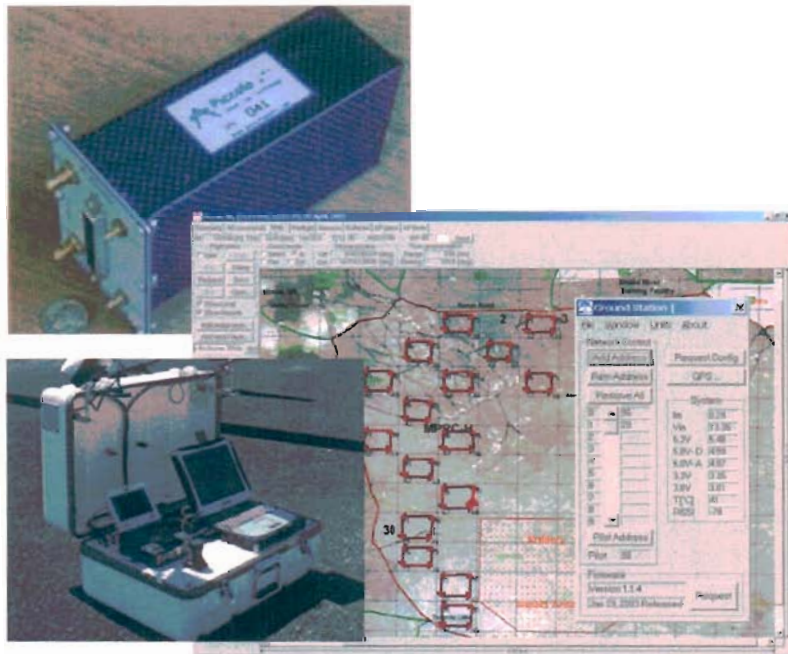
Figure 8: UAV Autopilot and portable ground control station.
