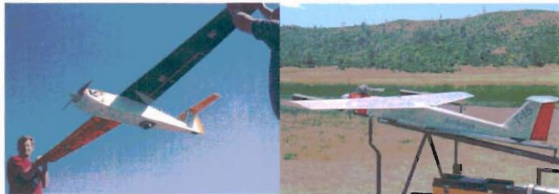
Figure 9: Arcturus-UAV T-15 fixed wing UAV on automated launcher and gimbaled camera system.
