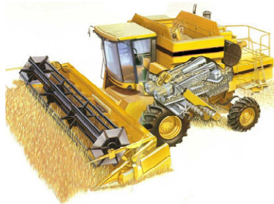
Figure 1: A modern grain combine represents the state-of-the-art in biomass separations.
