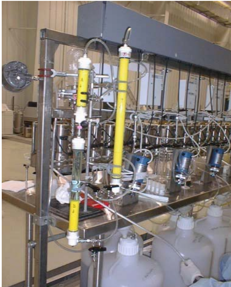
Figure 1. Ion exchange equipment used for AMP-PAN testing in the integrated flowsheet.
