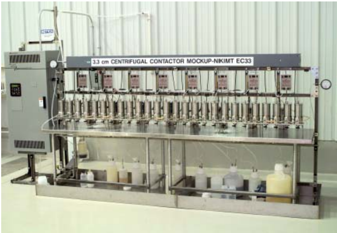
Figure 2. Centrifugal contactors used for the TRUEX and SREX solvent extraction flowsheets.
