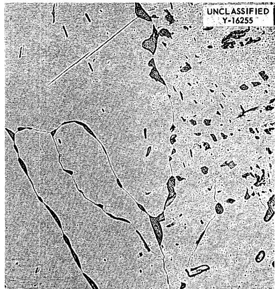
Fig. 132. Microstructure of the Region of Maximum Beta Phase in Zone-refined Zirconium Bar After Annealing at 860°C. Etchant: 60 parts lactic acid, 40 parts HNO 3 , and 4 parts HF. 50X. Reduced 17%.
