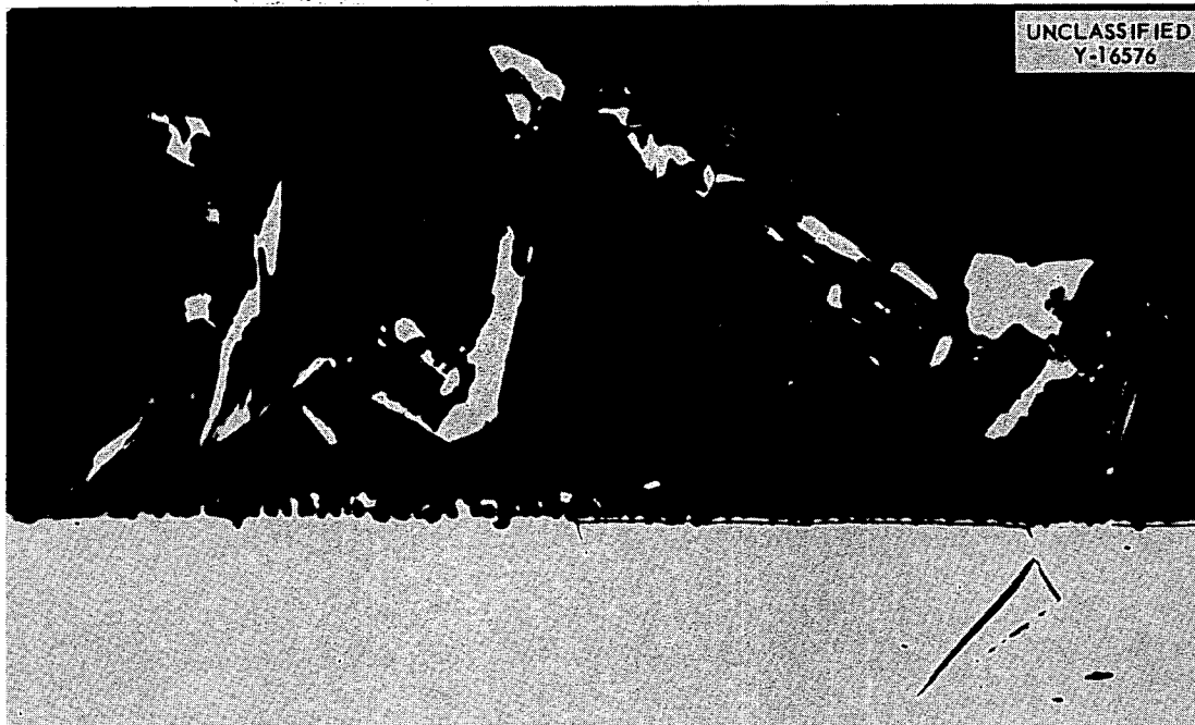
Fig. 71. Section of Nickel Cold Finger After Exposure to Fused Sodium Hydroxide Under a Blanketing Atmosphere of Hydrogen. The difference in magnitude of the mass-transfer deposits, on the surface at the gas-liquid interface and on the immersed surface, is illustrated. 100X.
