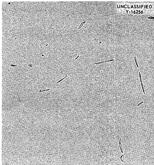
Fig. 130. Microstructure of Unpurified Portion of Zone-refined Zirconium Bar After Annealing at 860°C. Alpha and beta phases are shown. Etchant: 60 parts lactic acid, 40 parts HNO 3 , and 4 parts HF. 50X. Reduced 17%.
