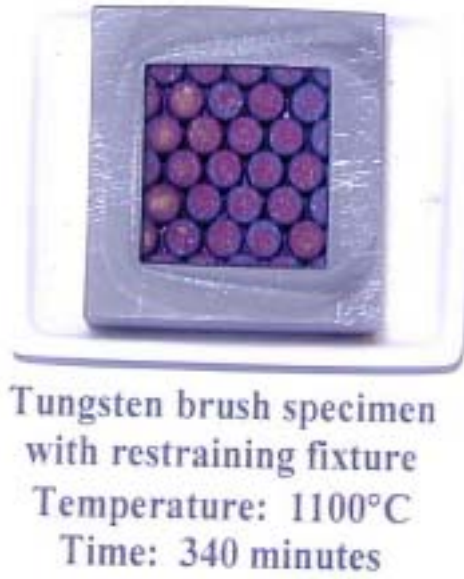
Figure 13. Tungsten brush specimens with restraining fixture tested at 1000 and 1100°C.
