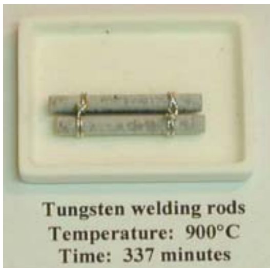
Figure 11. Photographs of tungsten rods tested in steam at 800, 900 and 1000°C.
