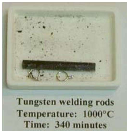
Figure 11. Photographs of tungsten rods tested in steam at 800, 900 and 1000°C.
