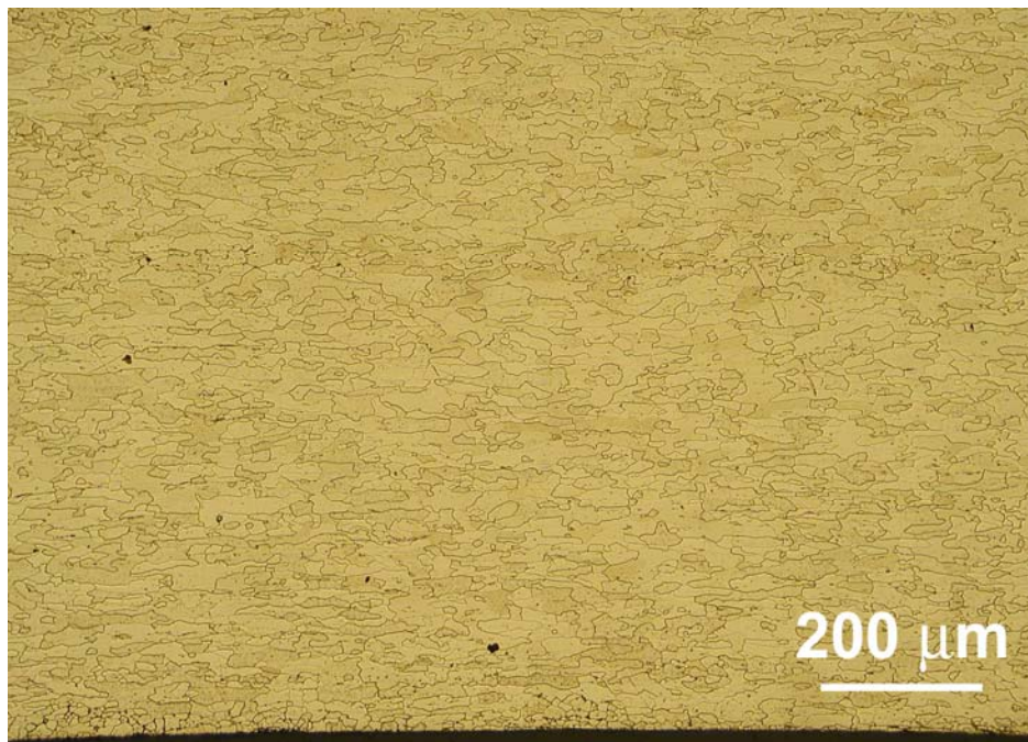
Fig. 14: Recrystallized grain structure near rolling surface of spray-rolled 2124. Sample was solution heat treated (493°C, 2 h.), cold rolled 75%, and annealed (493°C, 10 min.). Longitudinal section.
