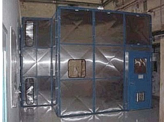
Figure 8. Permacon™ enclosure in which the Tritium Plasma Experiment is housed.
