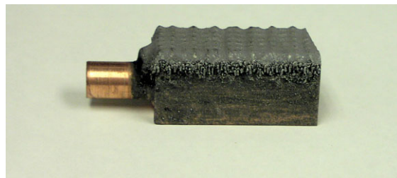
Figure 3. Plasma sprayed beryllium 5 mm thick on test specimen for the EFDA Project.
