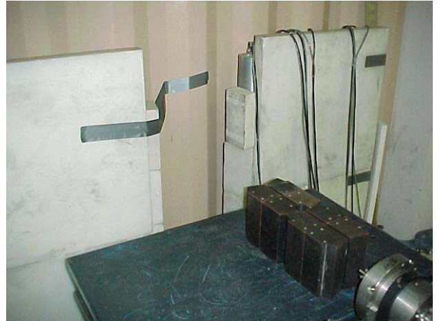
Figure 8. Side detector group with and without borated-polyethylene back shielding.
