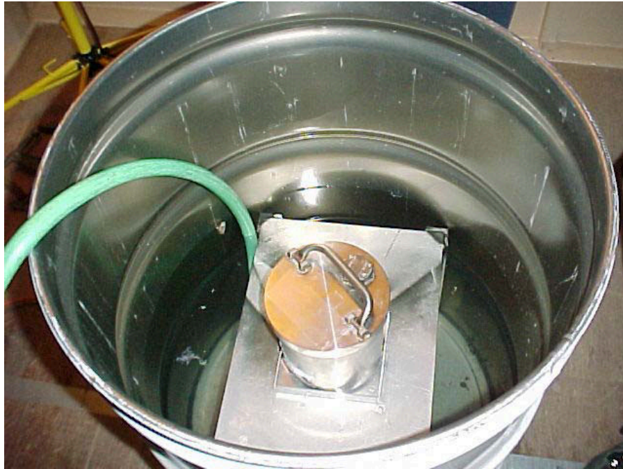
Figure 19. The top view of the water-filled, 55-gallon drum. The circular inner container (shown with a handle) was used to provide a watertight seal for the nuclear materials.
