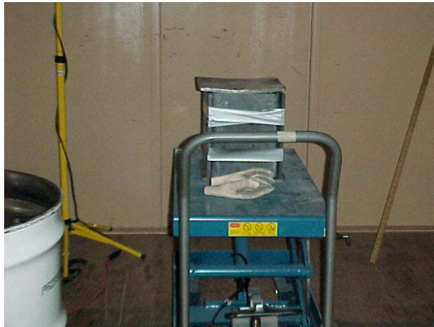
Figure 11. 1.27-cm thick lead shielding configuration used to shield nuclear material. Each lead shield side was approximately 30-cm square.
