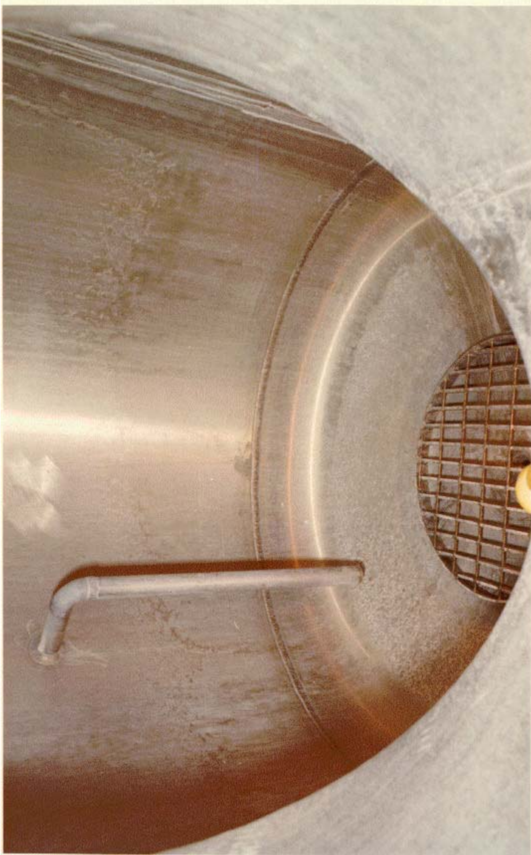
Figure A-18. View of the lower portion of mist eliminator (VES-NCC-110) before decontamination showing no calcine accumulation. The catch plate over the liquid drain line is in the lower part of the photograph (81-5568).
