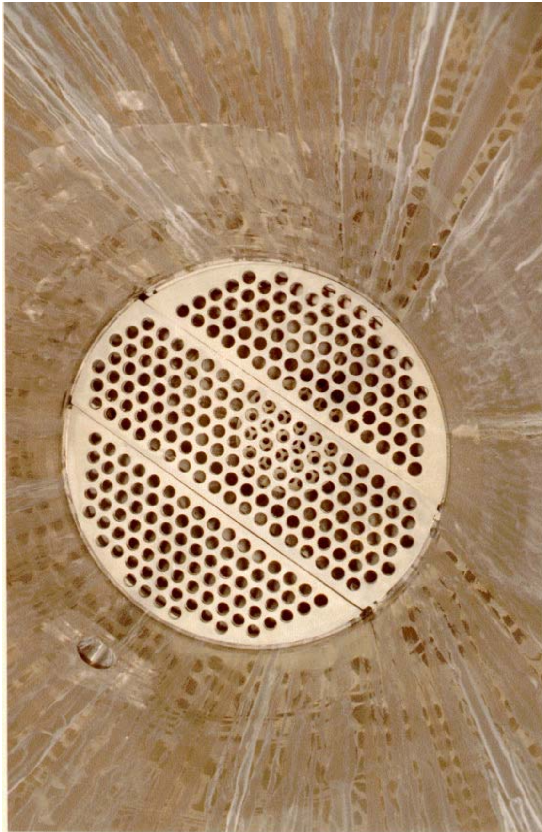
Figure A-14. Lower portion of the quench tower. The vessel was relatively clean prior to decontamination. Some streaks of dried quench solution residue are visible on the walls (81-5564). The Calcliner off-gas distribution plate is visible in the bottom of the vessel.
