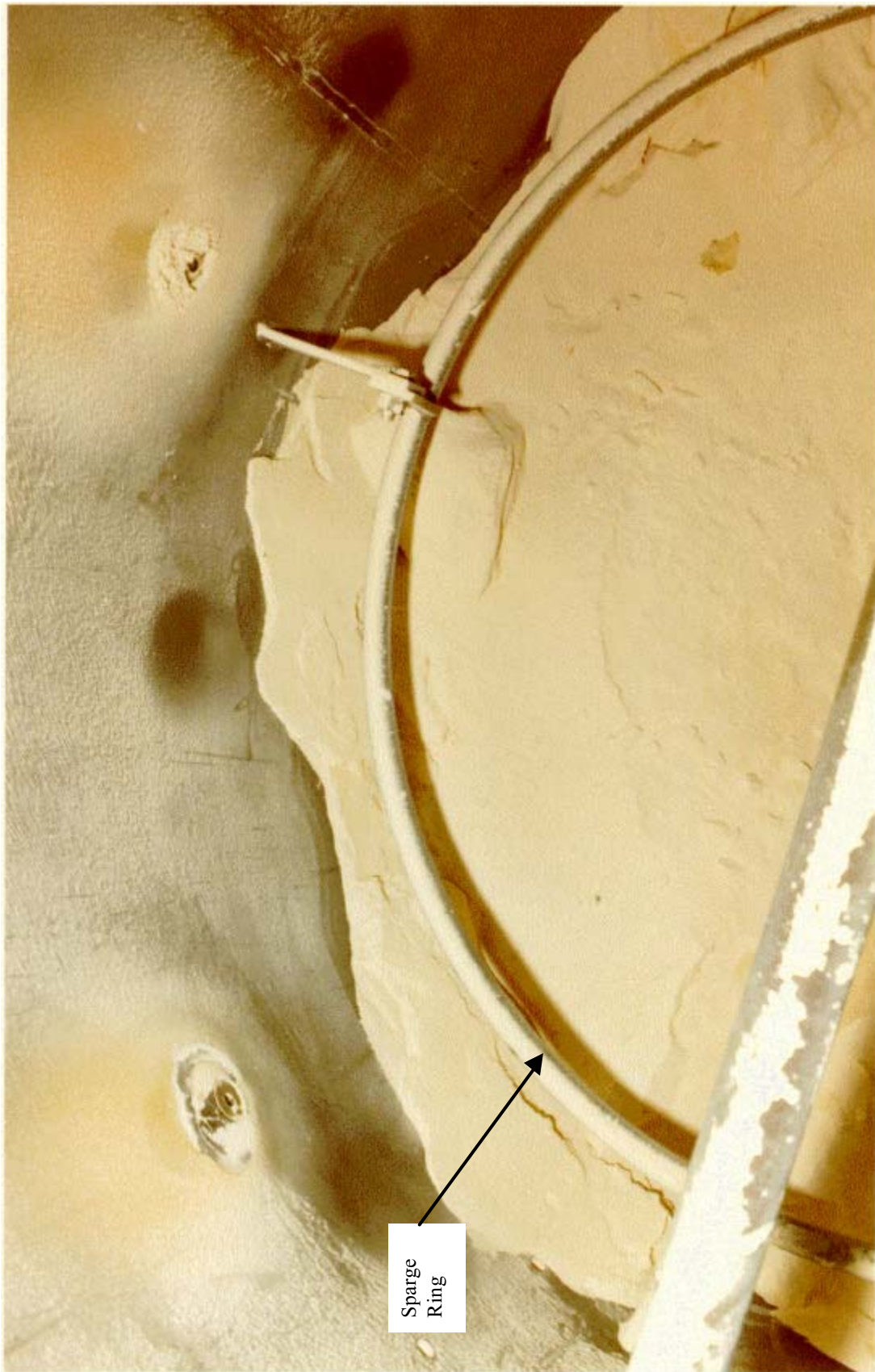
Figure A-8. View of the calcine remaining on the fluidizing air distributor plate following the June 1982 shutdown and before any decontamination. The calcine remaining on the distributor completely covers the fluidizing air distributor caps, but the sparge ring is visible above the calcine (82-4803).
