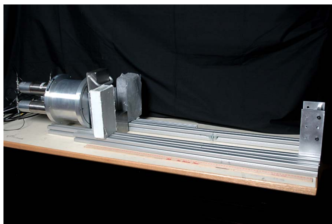
Fig. 5 A photograph of the optical rail system configured for testing of the Compton suppression detector assembly (at the far left.) The fixture attached to the rail at the far right of the photo is the aluminum source holder.
