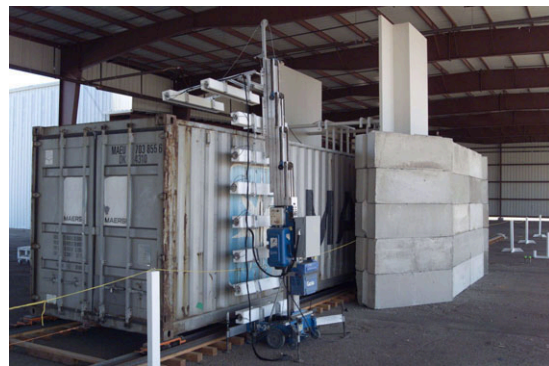
Figure 1. Deployed PPA detector assembly.
